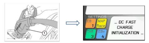
You can perform the DC charging with Power On (Key On) or Power Off (Key Off) motorbike status.
